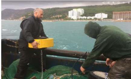
The deployment of the Wave Droid from the deck of a fishing vessel
